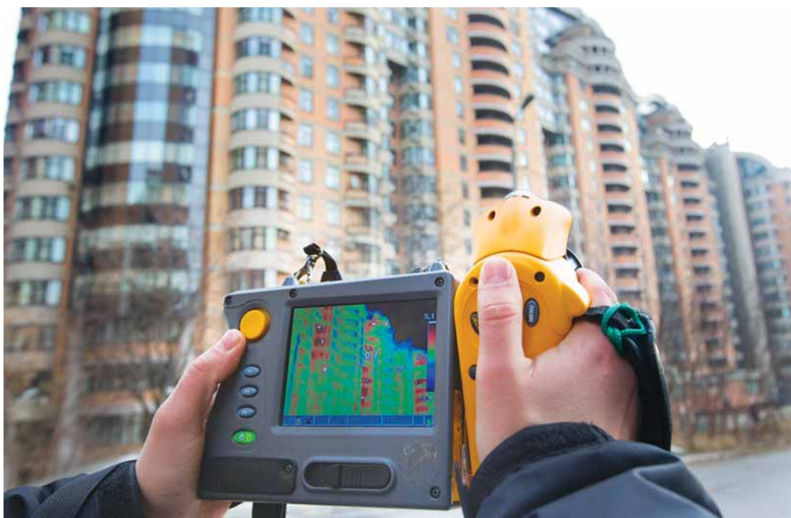
A worker measures the heat loss from a residential apartment block in Kyiv. Work to stimulate investment into making such buildings energy efficient across the country is being undertaken by the government with support from international development agencies. According to official figures, some $90 billion is needed for residential and municipal sectors -- 90 percent of the nation's annual gross domestic product. (Ukrafoto)
