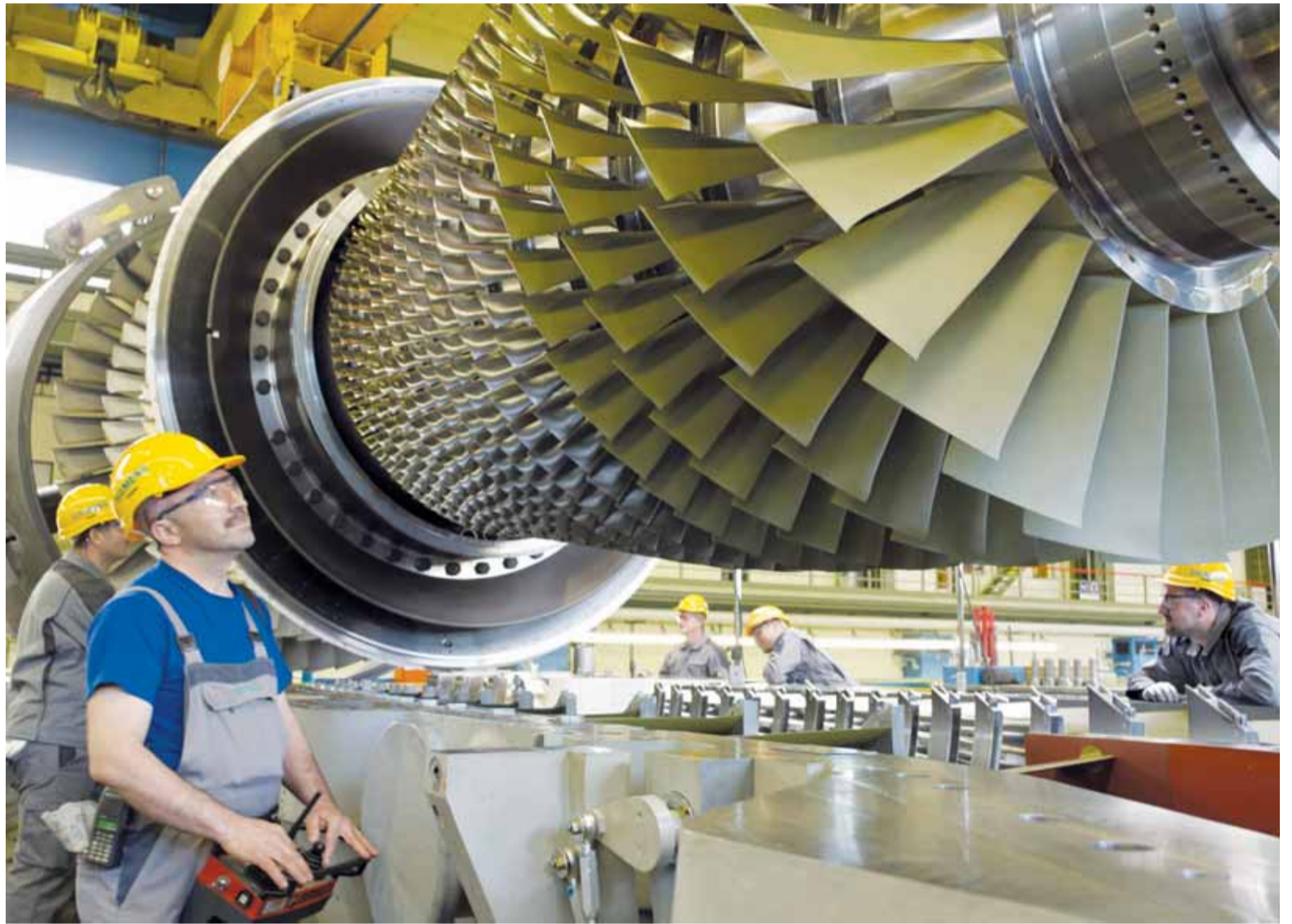
Siemens AG corporation employees insert a turbine rotor to the gas turbine SGT5-400F in a Siemens manufacturing plant in Berlin. (Siemens AG)
