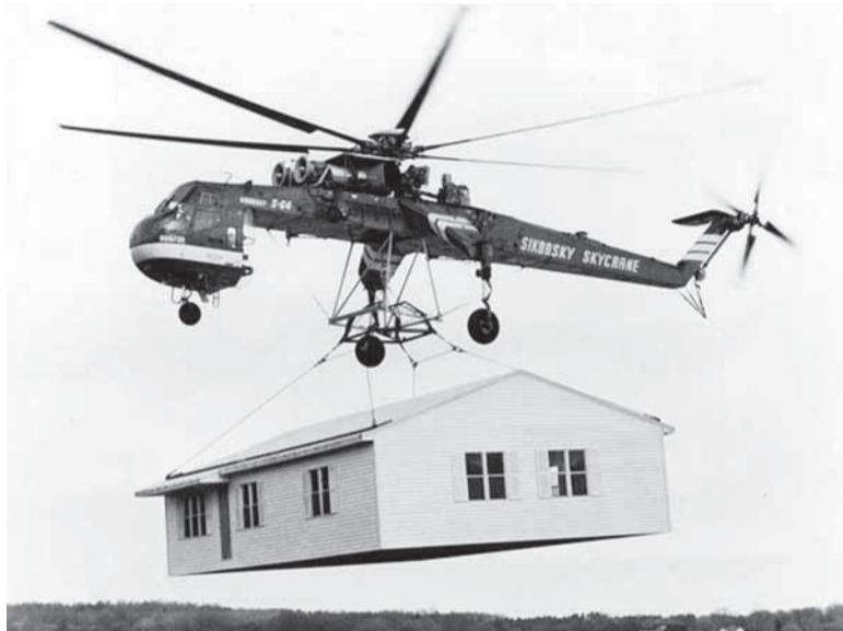
The Sikorsky S-64 Skycrane cargo helicopter is lifting a house. The machine was designed by Sikorsky Aircraft as a civil version of the CH-54 Tarhe for the United States Army in 1962. The current version of the heavy-lift helicopter is made by the Erickson Air-Crane company. (Courtesy)
