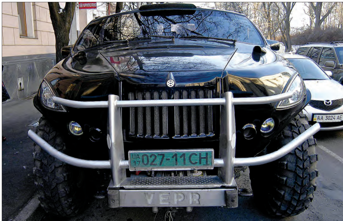
A heavily armored VEPR-S off-road vehicle seen in Kyiv Jan. 11. The VEPR-S is the first Ukrainian armored car for transporting money and other valuables. It weighs 6,500 kilograms and can carry 2,000 kg of cargo. (UNIAN)
