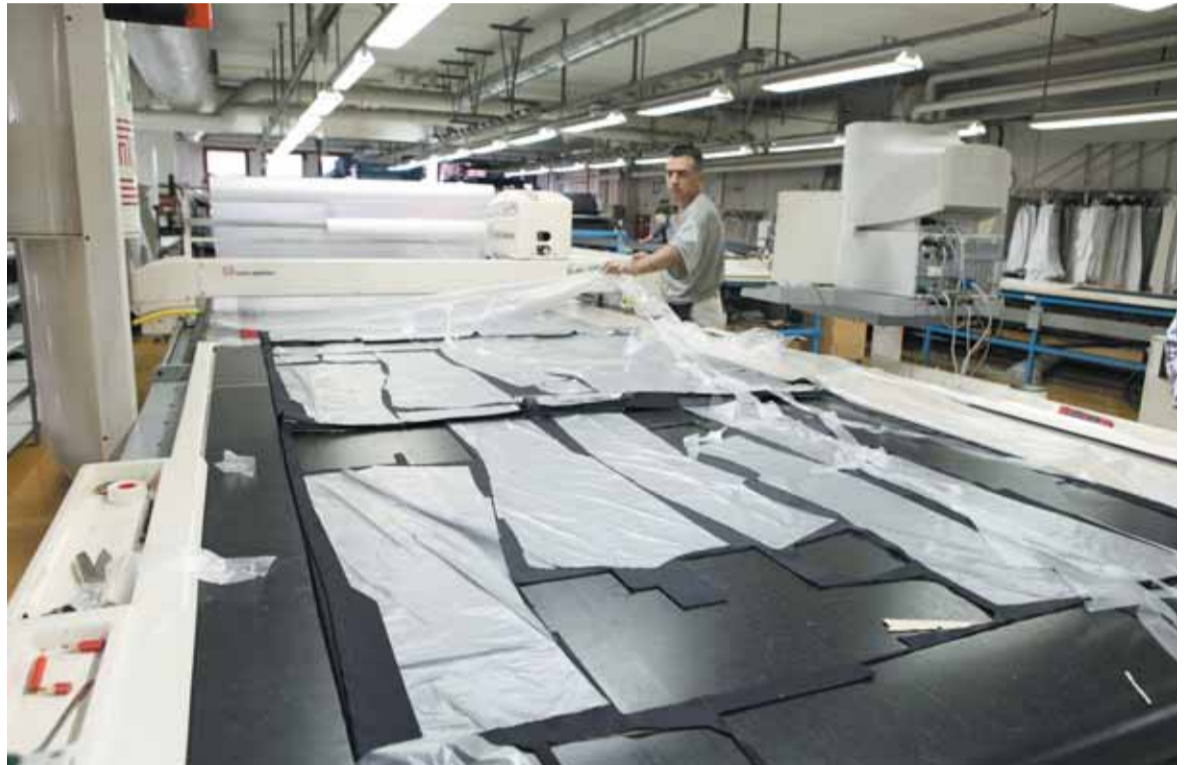
Cutting machine shapes details of future men's suits at Voronin factory in Kyiv. (Ganna Bernyk)
